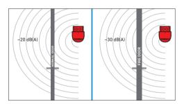
Decibel loss occurs through doors: approximately -20 dB(A) through a normal door, and approximately -30 dB(A) through a fire door. Unless a sounder is installed in a bedroom, it is unlikely that 75 dB(A) will be achieved.
