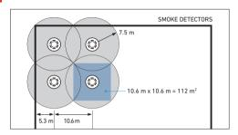
When mounted on a flat ceiling, smoke detection devices have an individual coverage of  $7.5 \,\mathrm{m}$  radius. However these radii must overlap to ensure there are no 'blind spots'. Therefore individual coverage can be represented by a square measuring  $10.6 \,\mathrm{m} \times 10.6 \,\mathrm{m}$  giving an actual area coverage of  $112 \,\mathrm{m}^2$  per device.
