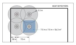
When mounted on a flat ceiling, heat detection devices have an individual coverage of  $5.3 \,\mathrm{m}$  radius. However these radii must overlap to ensure there are no 'blind spots'. Therefore individual coverage can be represented by a square measuring  $7.5 \,\mathrm{m} \times 7.5 \,\mathrm{m}$  giving an actual area coverage of  $56.3 \,\mathrm{m}^2$  per device.
