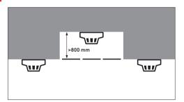
Voids less than 800 mm in height need not have independent coverage, unless fire or smoke is able to spread from one area to another through the void or risk assessment shows AFD (Automatic Fire Detection) to be necessary.
