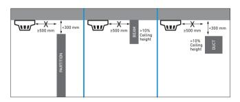
A device should not be mounted within 500 mm of any obstruction.
