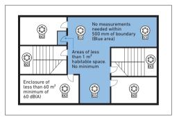
The minimum sound level should be 65 dB(A) or 5 dB(A) above a background noise which is louder than 60 dB(A) (if lasting more than 30 seconds) and at a frequency of between 500 Hz and 1000 Hz. The maximum sound level should not be greater than 120 dB(A) at any normally accessible point. May be reduced to 60 dB(A) in stairways, enclosures up to 60 m² and specific points of limited extent. If using fire alarm as as lockdown alarm this must be a distinctly different tone to that of the fire alarm.
