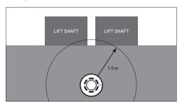
Vertical shafts like lifts, risers and open stairways should have a device mounted within 1.5 m of any opening. (This is not necessary for enclosed stairways, because as noted below, there are detectors on every landing within the stairway).
