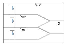
Enclosed stairways should have a detector at the top of the stairway and on each main landing.
