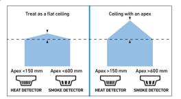
For ceilings that feature an apex: as long as the height of the apex from the rest of the ceiling is less than 150 mm for heat detectors or less than 600 mm for smoke detectors, then these can be treated the same as flat ceilings. For higher apexes, a device should be installed at the highest point. The distance to adjacent devices can be increased by 1% per degree of angle of the roof up to a maximum of 25%.
