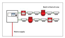
Fire resistant cabling is now required within the whole fire alarm system including the mains supply cables. The use of non-fire resisting cables whether mechanically protected by fire-resisting construction or not, will no longer comply with BS 5839-1. All detection, alarm and mains supply FR cables should be red in colour.
