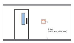
The centre of the element of the manual call point should be positioned 1.4 m (+/-300 mm) from floor level. Unless a wheelchair user is likely to be the first person to raise the alarm. (Between 800-1200 mm according to Doc. M. + Equality Act). BS 5839 states transparent hinged covers should be fitted to all manual call points.
