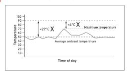
The minimum static response to heat devices should not be less than 29°C above the average ambient temperature, or less than 4°C above the highest temperature the device can expect to experience.
