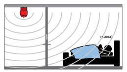
For areas where people are sleeping, sounder devices should produce a minimum 75 dB(A) at the bed-head with all doors shut. In buildings providing sleeping accommodation for deaf or people with impaired hearing, bedrooms should have both audible and visual alarms. (Note: Visual Alarm Devices are not intended to wake sleeping persons).
